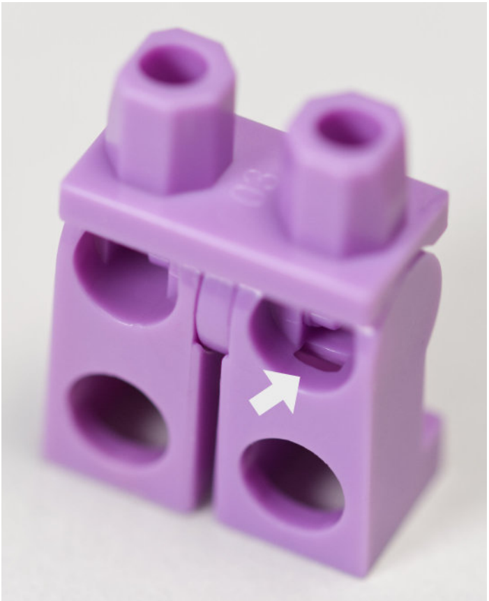
The through-hole molded only into the right leg.
