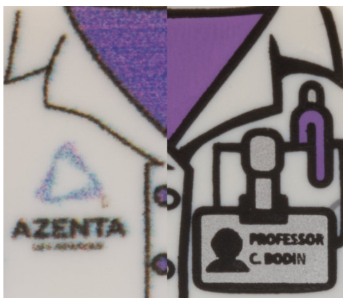
Clone torso left and LEGO torso right. Note the stipple pattern nature of the composite colors on the clone. The purple of the clone shirt is composed of blues and magentas while the LEGO purple is solid purple. Clone blacks have a color halo around them and rough edges where LEGO black is black and has a crisp edge.
