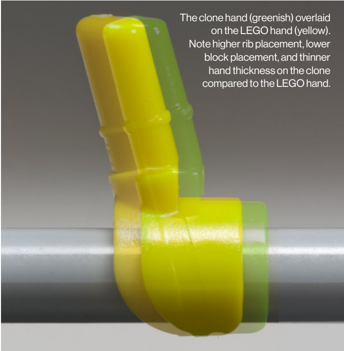
A LEGO hand, left, and the clone hand, right. This particular LEGO hand has an angled terminus of the bar, digits on the dorsal side of the angular wrist block, and digits on the bar between the wrist block and the rib on the ventral side of the bar.
